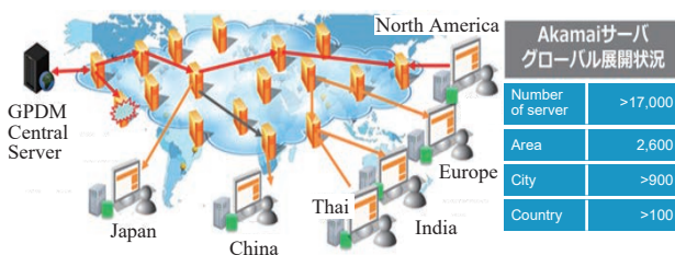
Fig. 2 Image of GPDM system structure with Akamai
