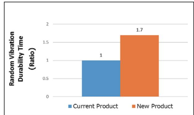
Fig. 4 Vibration Durability
