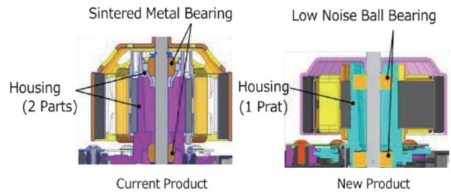
Fig. 3 Comparison of Motor Structure
