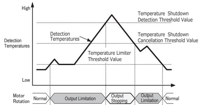
Fig. 7 Timing Chart of Over Temperature Protection
